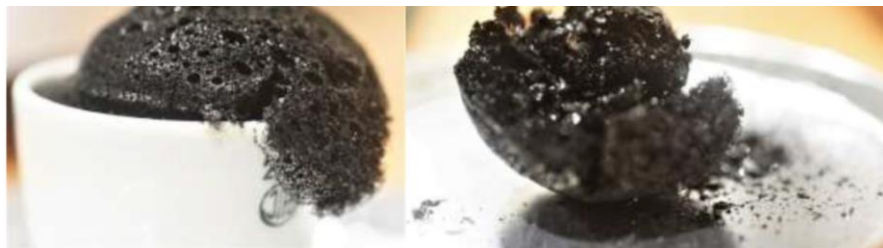
Figure 4. Pictures of birch lignin after carbonisation at the higher temperature of the range selected
