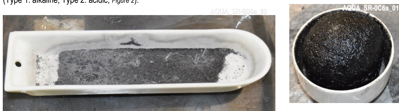
Figure 2. Pictures of S. ramosissima lignin after activation with 2 different types of agents
