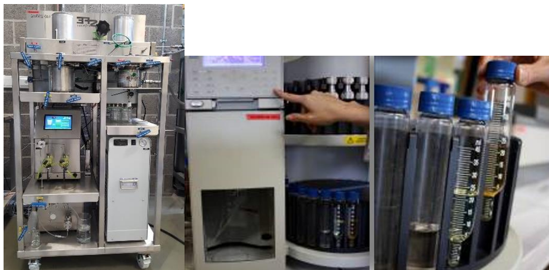
Figure 5: Lab-scale devices at CEL for the extraction by supercritical CO 2 (SFE 100ml lab station at the left) and subcritical water (Dionex ASE350 at the right).
