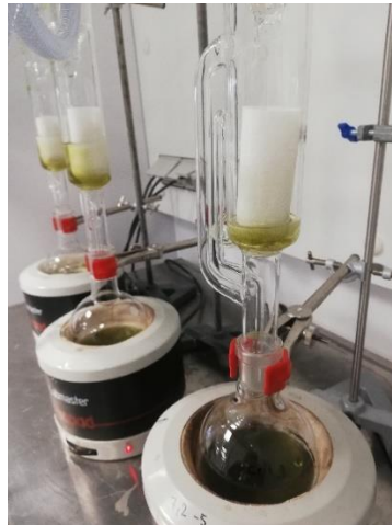
Figure 4: Extraction of C. maritimum fibre residue with Soxhlet.
